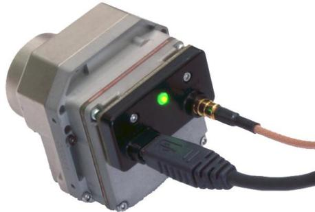
**Figure 3: VPC Physical Connections**
